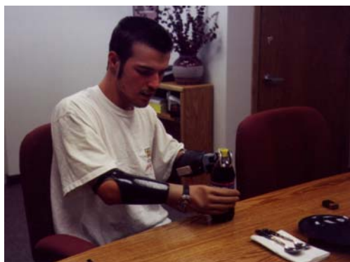
Figure 3 The electric hand and the Synergetic Prehensor may be used together effectively, as in this example, the hook providing better purchase
